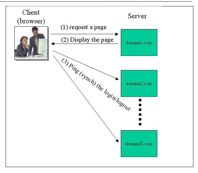
In the figure above, we illustrate the concept of the ping (or synchronization) of the login and logout.
